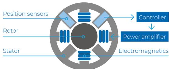
Active magnetic bearings – Five axis active bearings utilize two coils each for precision placement that keeps true rotor placement integrity.
