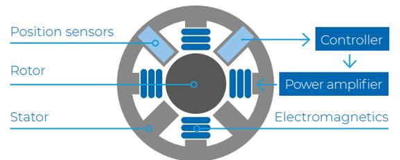
Active magnetic bearings – Five axis active bearings utilize two coils each for precision placement that maintains rotor position with micrometer accuracy.
