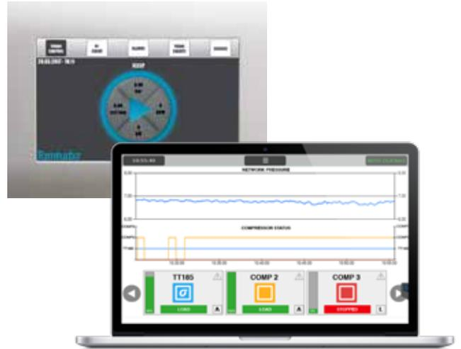
PLC based controller has a touch screen user interface for local or remote monitoring and operating the unit.
