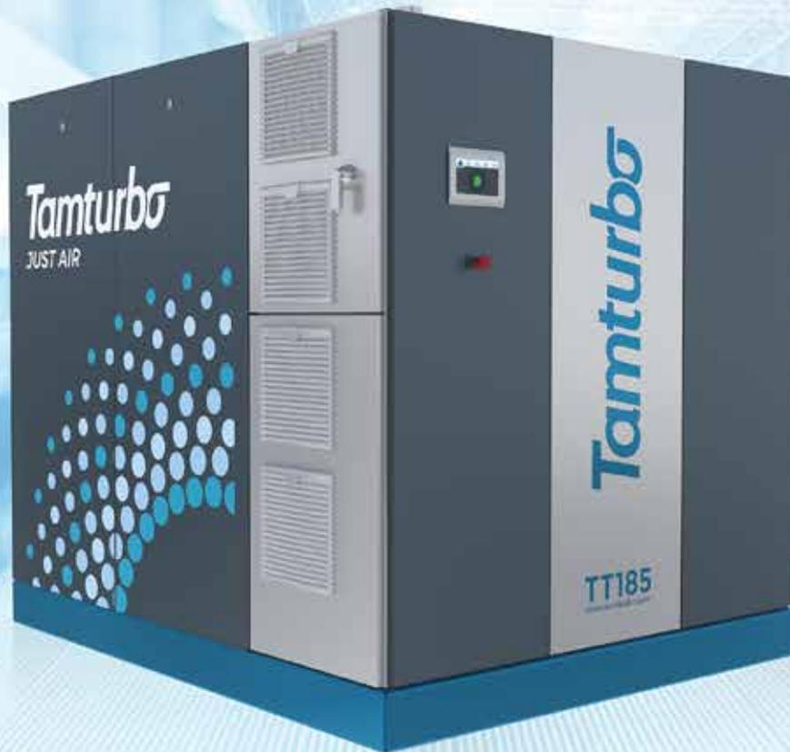
**ALL TAMTURBO® TOUCH-FREE™ COMPRESSORS** are Variable Speed-controlled, direct driven high-speed turbo compressors that produce completely oil-free compressed air for industrial customers. Impellers are integrated directly on the motor shaft without any couplings.
